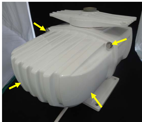
23) Attach the back cover by tightening four fixing bolts. (Tool: Wrench 13mm)
