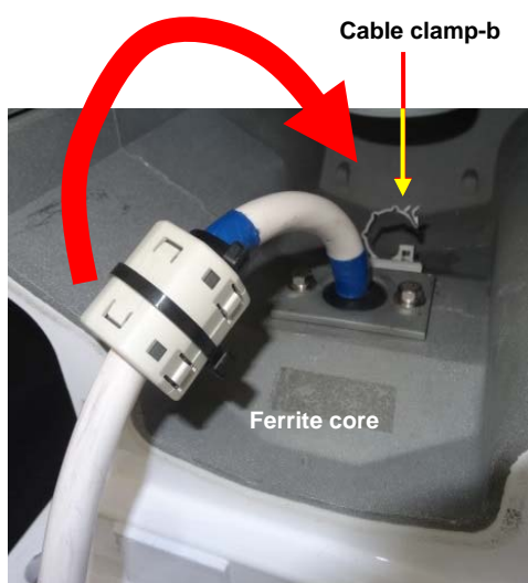
13) Tilt the cable with the ferrite core toward the cable clamp-b.
