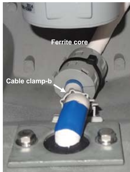
14) Clamp the cable by the cable clamp-b.
