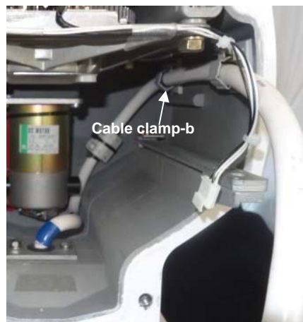
14) Clamp the cable by the cable clamp-b.
