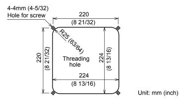
Fig. 5.5 Work of fiush-mount installation hole
