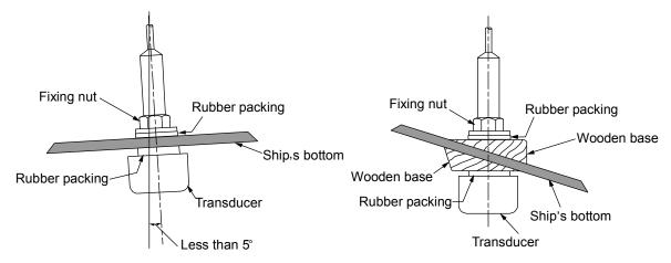
In case that the slope of ships bottom is less than 5°
