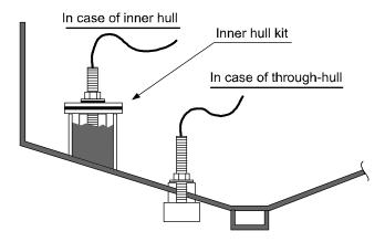
Figure 5.6 Installation of Transducer
