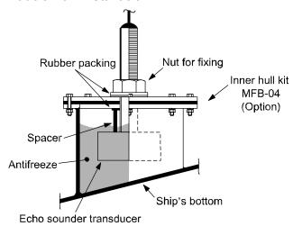
Figure 5.7 Inner-Hull installation
