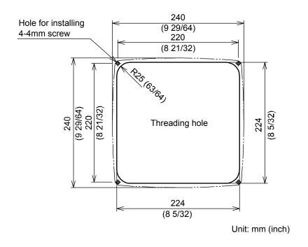
Dimension drawing of flush-mount installation
