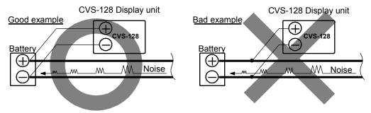
Fig. 5.1 Connection of Power Line
