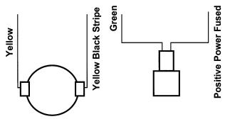
**Reversing Motor and Bypass Valve Connections**
