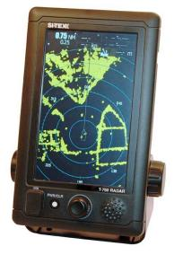
The T-760 Series case measures only 5.4" W X 8.9" H X 3.5" D. Yet, this system boasts a long list of professional-grade features, including powerful 4kW output, up to 48nm range, multi-speed antenna rotation, standard 50-target AIS tracking capability and standard 10-target MARPA — features often associated with larger, costlier systems. Control of all these features is achieved via the T-760's touch screen LCD display and single rotary encoder dial, for simple, intuitive operation.
