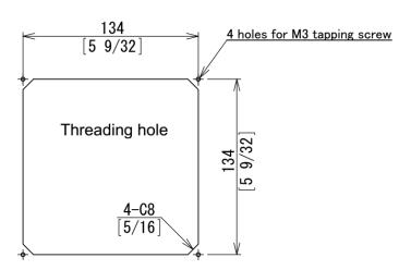
Figure 7.3 Flush Mount installation
