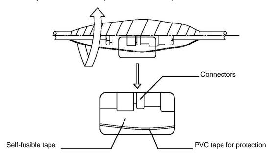
Figure 7.5 Processing on the coax cable jointing section
