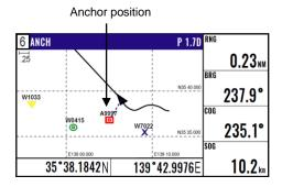
**RNG**: Distance from anchor position. **BRG**: Bearing from anchor position.
