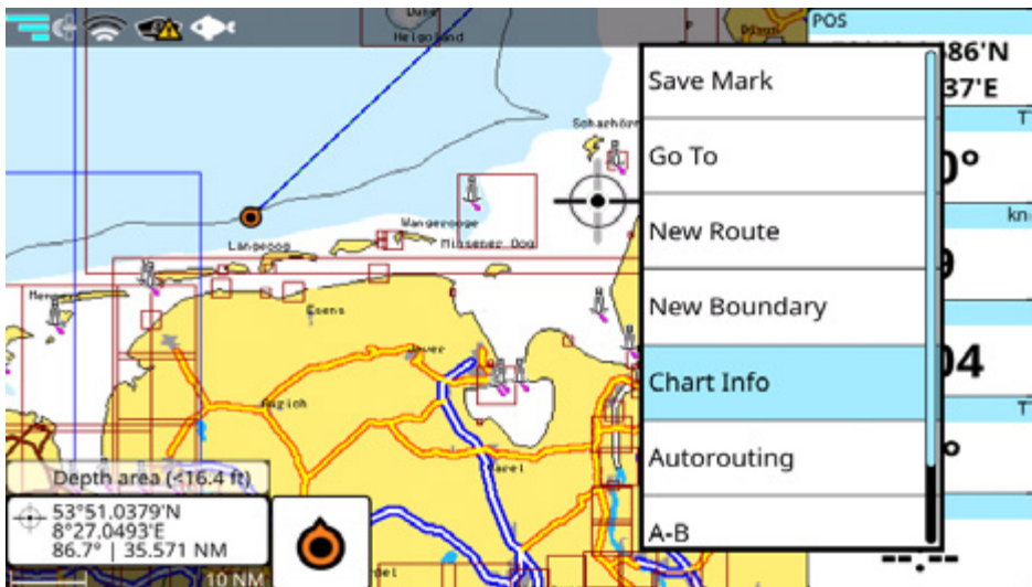
Figure 5.3 - Object's Quick Info popup and Chart Info contextual menu on the Map page
