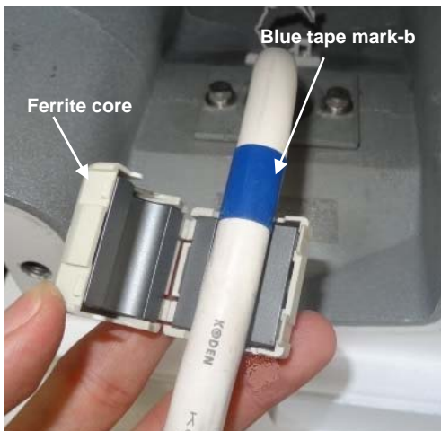
11) Attach the ferrite core to side of the blue tape mark-b.
