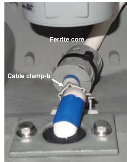
14) Clamp the cable by the cable clamp-b.
