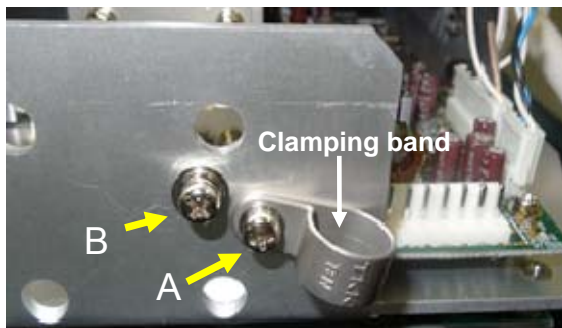
20) Remove screw-A and screw-B.
