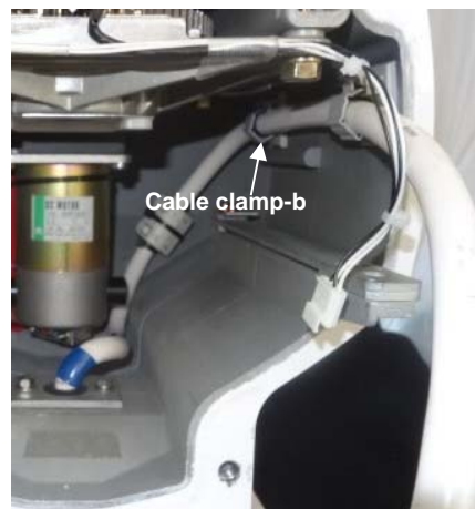
14) Clamp the cable by the cable clamp-b.
