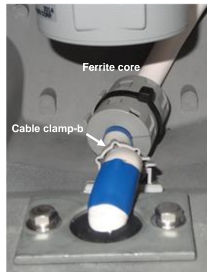
14) Clamp the cable by the cable clamp-b.
