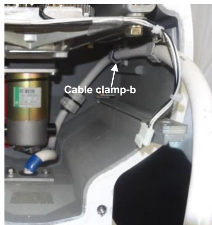
14) Clamp the cable by the cable clamp-b.
