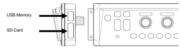
Fig.1.32 Connection of USB Memory and SD Card
