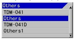
When [Others] is selected, one kind of high-frequency and one kind of low-frequency can be set up.
