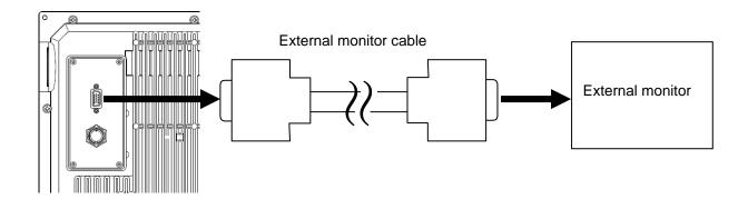
Fig. 1.30 Connection of External Monitor-2
