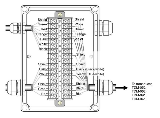
Fig. 1.26 Connection between junction box and transducer
