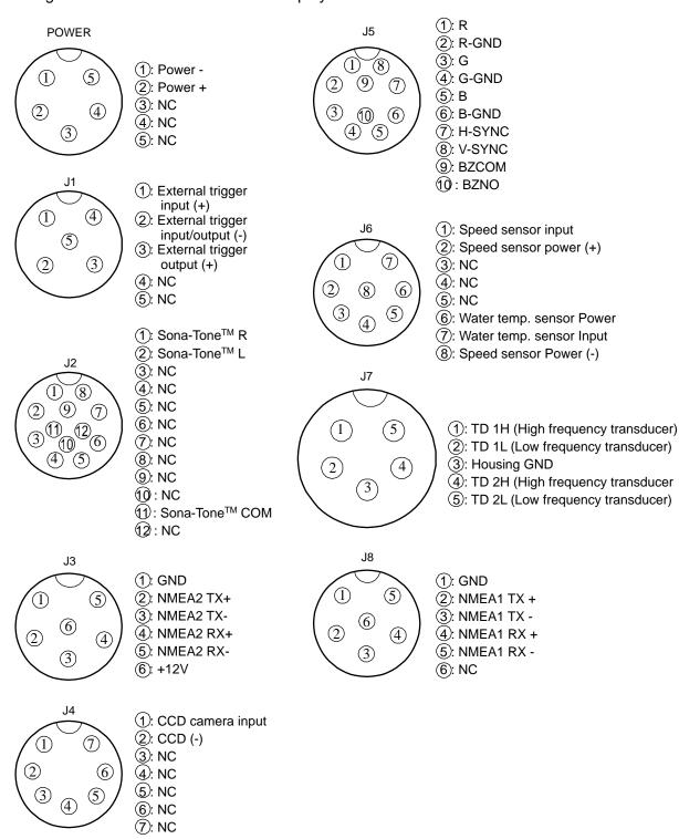
Fig. 1.20 Pins assignment of rear connector-1
