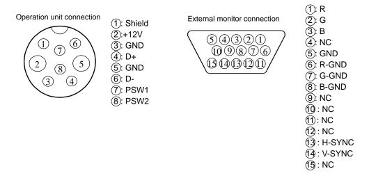
Fig. 1.21 Pins assignment of rear connector-2
