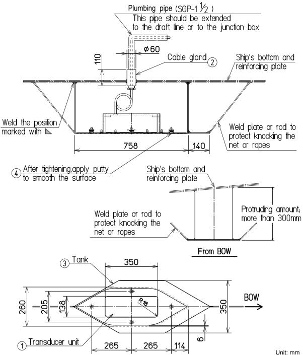
Fig. 1.13 Mounting of a transducer on steel boat (For Anti-resonance)
