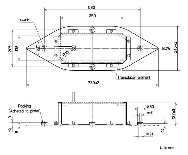
Fig. 1.14 Outline view of a transducer unit on steel boat (For Anti-resonance)
