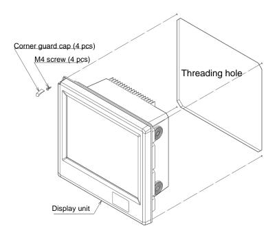
Fig. 1.4 Flush-mount installation
