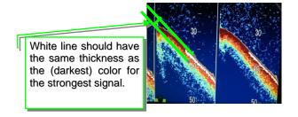
5. Pressing the gain knob at the side to be adjusted a few times, move to the position of the Gain (TD) box to be adjusted. (the red mark at right top side will move)
