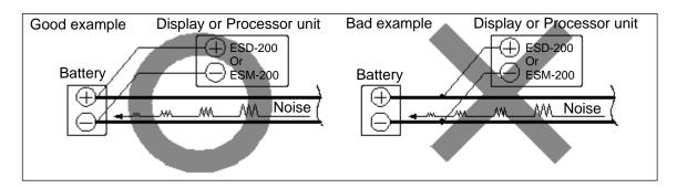
Fig. 1.1 CVS-FX2/FX2BB Connection of Power line
