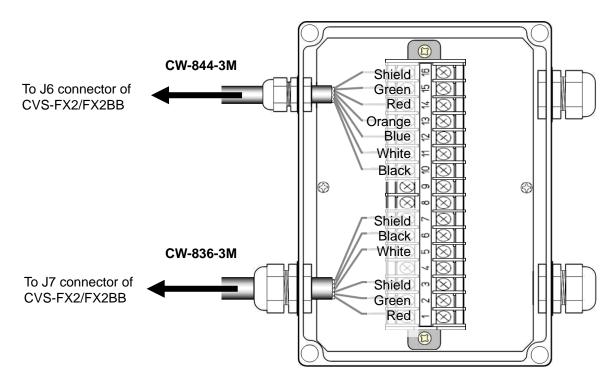
Fig. 1.24 Connection between CVS-FX2/FX2BB and junction box
