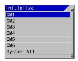
When an specified CM is to be initialized, select [CM1] to [CM6] with [▲] and [▼] keys. To initialize the whole system, select [System ALL].
