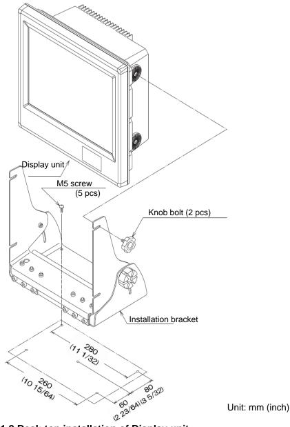
Fig. 1.2 Desk-top installation of Display unit
