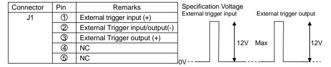
Fig. 1.27 External trigger
