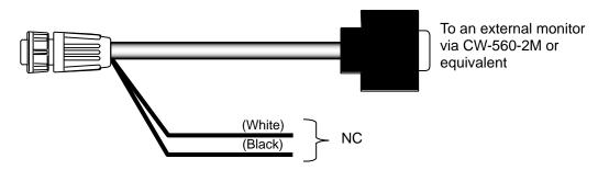
Fig. 1.29 Connection of External Monitor-1
