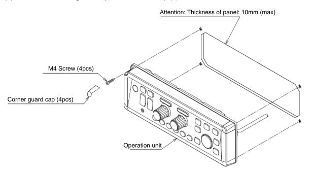
Fig. 1.9 Flush-mount installation of Operation unit
