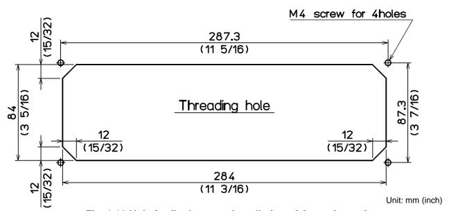
Fig. 1.10 Hole for flush-mount installation of Operation unit
