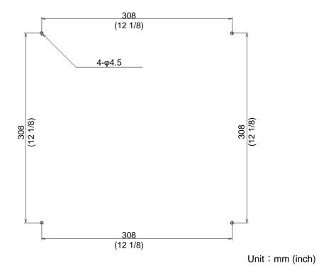
Fig. 1.6 Position of installation hole of Processor unit
