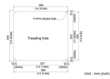
Fig. 1.5 Hole for flush-mount installation of Display unit
