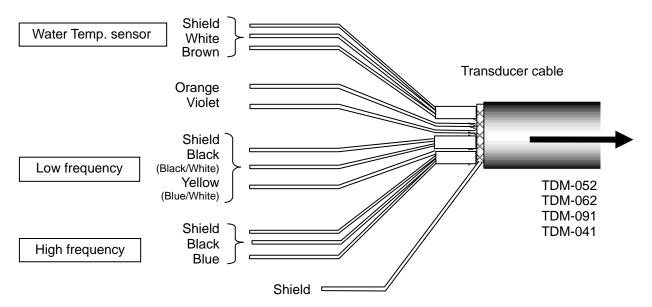
Fig. 1.25 Details of transducer cable
