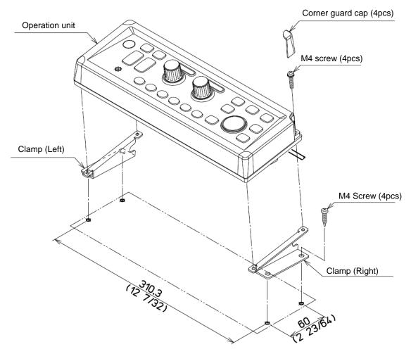
Fig. 1.7 Desk-top installation of Operation unit
