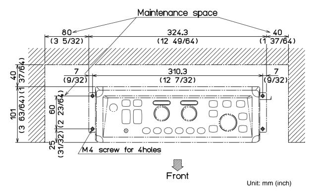
Fig.1.8 Maintenance space of desk-top installation
