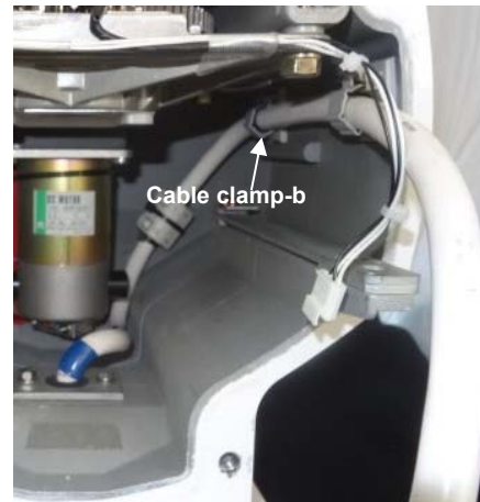
14) Clamp the cable by the cable clamp-b.
