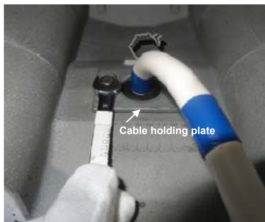
10) Attach cable holding plate and fix it with two bolts. (Tool: Wrench 8mm)
