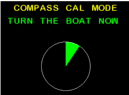
Figure 28: Start turning the boat clockwise at low speed, hold the turn.
